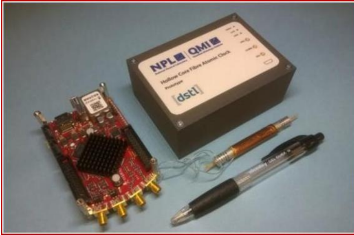
Figure 19: Enclosure, physics package and electronics of hollow core clock. Courtesy Professor Patrick Gill NPL
