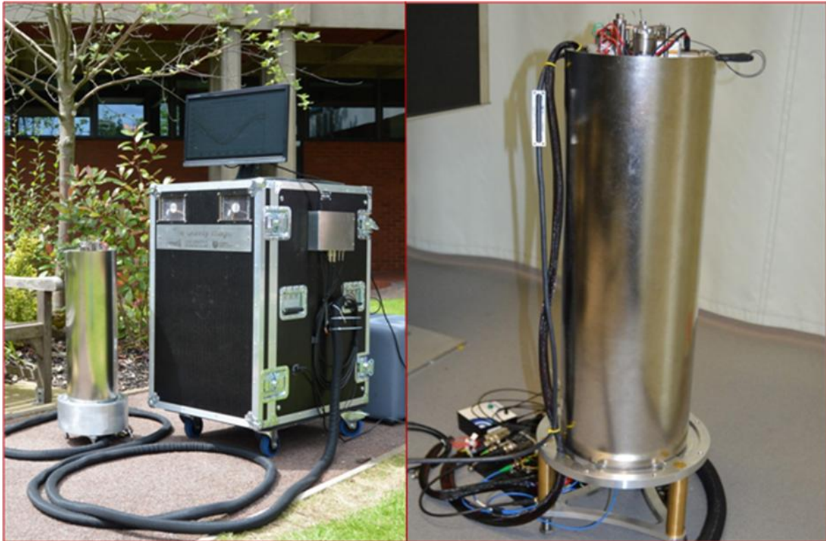
Figure 10: Portable atomic gravimeter demonstrator (right) and together with engineering test harness during field trials (left). A portable gradiometer is expected by the end of 2016. Courtesy of Mike Holynski, Birmingham University
